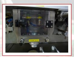
Standard options include integrated bottle blowing devices to clean bottles of debris and selected face orientation devices to consistently feed bottles to conveyor in specific direction.
