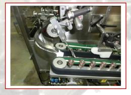
Once bottles are orientated a simple format hook will identify neck/base of bottle to orientate them so base of bottle is leading in readiness to be stood up and discharged onto the out-feed conveyor
